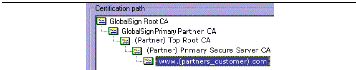
Figure 2: Certification Path - the new chain once a CA is RootSigned by GlobalSign
